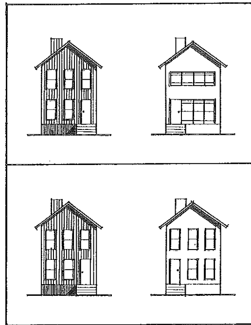
These two comparisons depict relationships between historic and new buildings in terms of the relationship of solids to voids. The upper example is that of a historic house (shaded) with evenly-spaced vertical sash windows standing next to a new building with large bands of glass resulting in a horizontal feeling even though the building itself is vertically oriented. The lower example shows a more compatible relationship of solid wall space to window and door openings on the new building.
